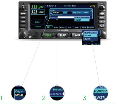
To begin the process of selecting a departure procedure, tap on the Origin box to select. A 'Departure' field will appear. Tap the 'Departure' field. A dropdown list of available departure procedures will be displayed. Select the transition (departure Runway) and push ENTR.
