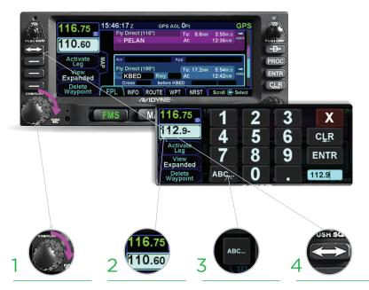
Use the COM/NAV knob. Push the knob to display NAV frequencies. Then, twist the inner knob to direct-tune got KHz and the outer knob to adjust MHz. Touch the standby frequency field to display the numeric keypad. Enter the desired frequency.
