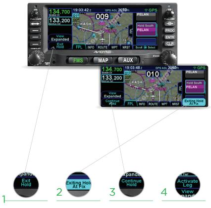
To Exit the hold, select the "Exit Hold" Line Select Kev (LSK1), and the FMS will exit the hold the next time it passes the hold fix.
