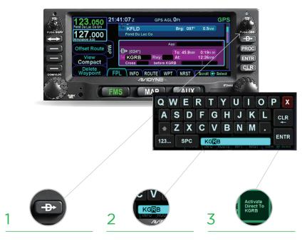
Press the Direct-To button to display a green Direct-To dialog box pre-populated with a logical waypoint (powered by Geofill™). **To enter a different waypoint,** tap the data field in the top dialog box. The QWERTY keyboard appears for you to enter the desired waypoint identifier. **To approve,** tap the 'Activate' dialog box to select. Pressing ENTR or the right knob can also be used to confirm.
