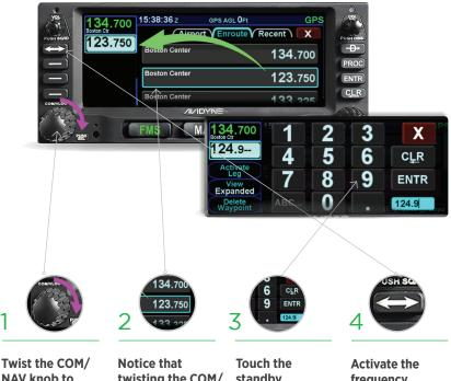
NAV knob to direct-tune. Use the inner knob for KHz and the outer knob to adjust MHz.
