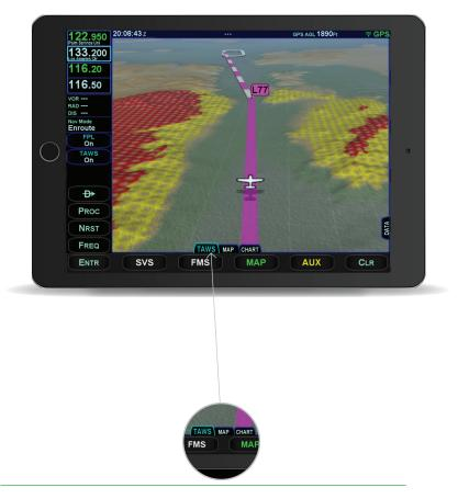
**Select the TAWS Tab on the MAP page of the IFD100 to view 3D Exocentric Synthetic Vision,** which includes 3D Terrain, Obstacles, Traffic (when available), Airports.
