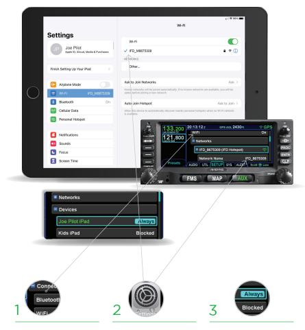
From AUX->SETUP page, double touch or highlight and push right knob to expand the +Connectivity menu. Set IFD WiFi to 'ON' using touchscreen or by turning inner right knob. Go to Settings Menu on iPad and select WiFi that matches your IFD's Network name. Enter Password shown under +Network menu. Then launch IFD100 App so that IFD sees that you are trying to gain permission to connect.
