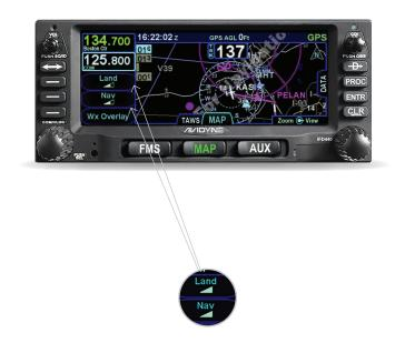
**To select the preferred level of map density displayed,** from the Map Page, Map tab, press the "Land" LSK to declutter the terrain base map and/or "Nav" LSK to declutter off-route NavAids (Intersections, Airports, VORs etc). There are four levels of declutter for each. The specified level of detail will remain consistent across all map pages. (Terrain Awareness alerts and nearby Traffic are not affected by declutter settings.)
