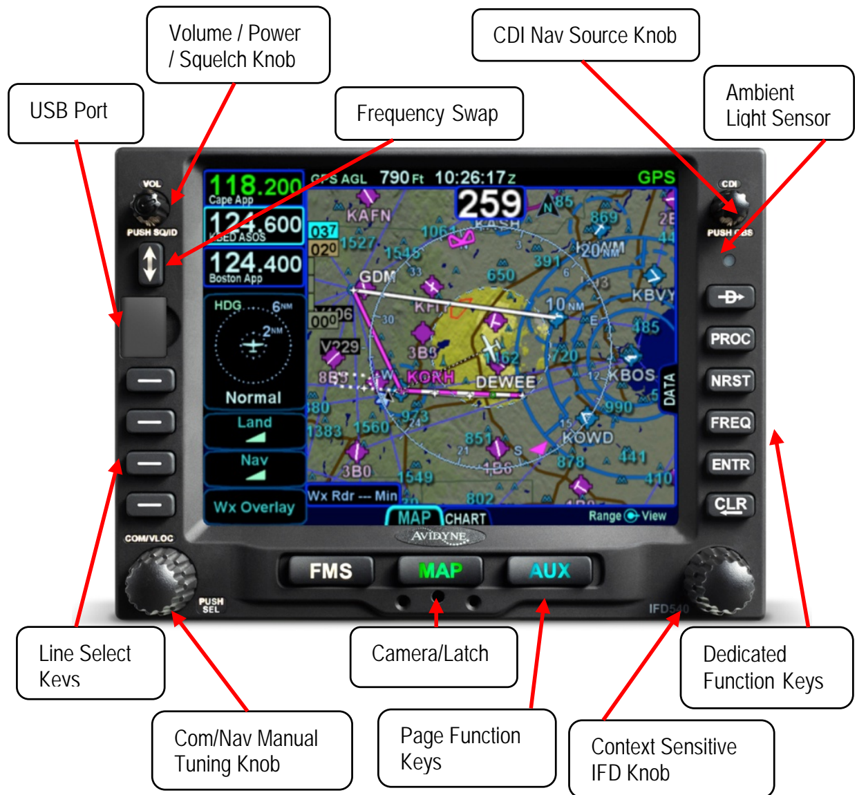
Figure 1. Avidyne IFD540 700-00182-XXX Integrated Flight Display (IFD).
