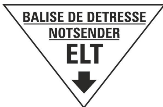
Figure 2-6 - Near the distress beacon.
