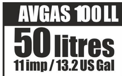
Figure 2-4 - Near the cap of the supplementary tank, if installed.
