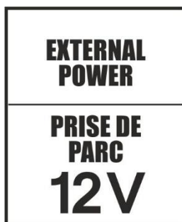
Figure 2-7 - On the access hatch of the ground power socket (if installed) on the starboard side of the aircraft.
