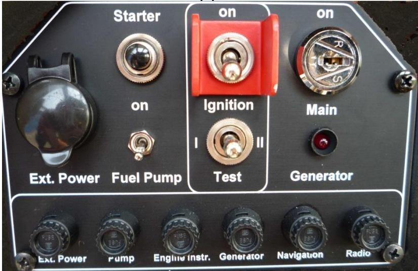
Ext. Power 2A    Pump 8A    Eng.Instr. 500mA    Generator 500mA    Navigation 2A    Radio 2A
