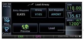
Touch to load selected airway to flight plan.
